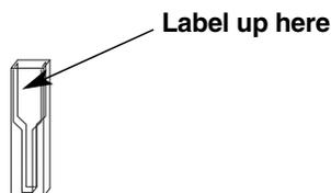
2. You must first “blank” the spectrophotometer. Load the S1 cuvette, close the door and hit the “0 ABS / 100% T” button. Now measure and record the absorbance for the remaining standards in Table 2 below.
